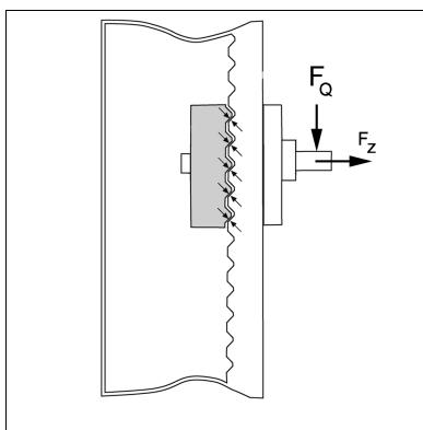
Note: The permissible load capacities of the channels are to be respected..
