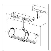
The permissible bending moment of the connection elements (threaded rod or threaded tube) may restrict the application!
