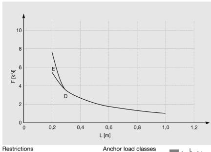
restrictions  $\sigma_{perm} \le 160 \text{ N/mm}^2$   $f_{perm} \le L/100 \text{ for } L > 300 \text{ mm}$   $f_{perm} \le 3 \text{ mm for } L = 200 \dots 300 \text{ mm}$
