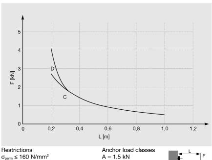
Restrictions  $\sigma_{perm} \le 160 \text{ N/mm}^2$   $f_{perm} \le L/100 \text{ for } L > 300 \text{ mm}$   $f_{perm} \le 3 \text{ mm for } L = 200 \dots 300 \text{ mm}$
