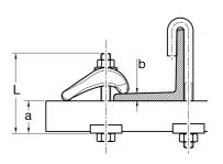
M12:  $L_{min} = a + b + 47$  [mm] M16:  $L_{min} = a + b + 57$  [mm]
