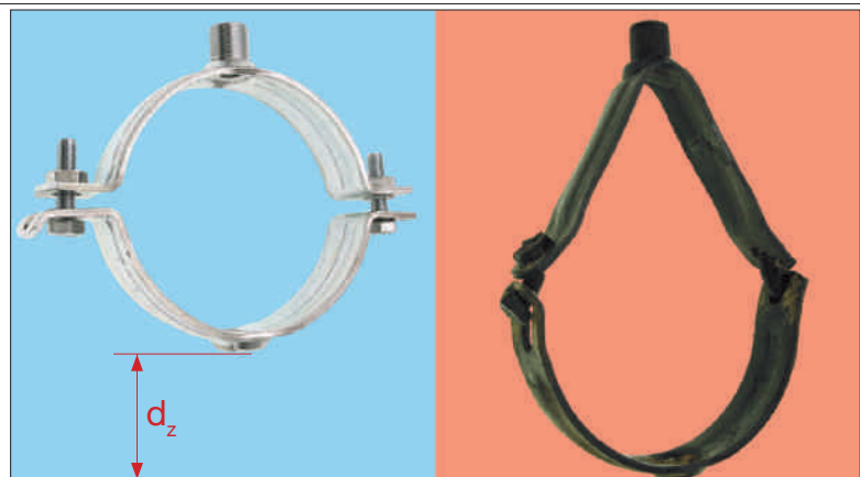
Figure 6.3: Stable D-3G pipe clip before and after the fire test / Sikla
